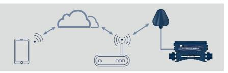
Power Supply : DC12V Max 200mA Frequency : 2.4GHz Wireless Standard : IEEE 802.11 b/g/n Working Model : AP/STA
